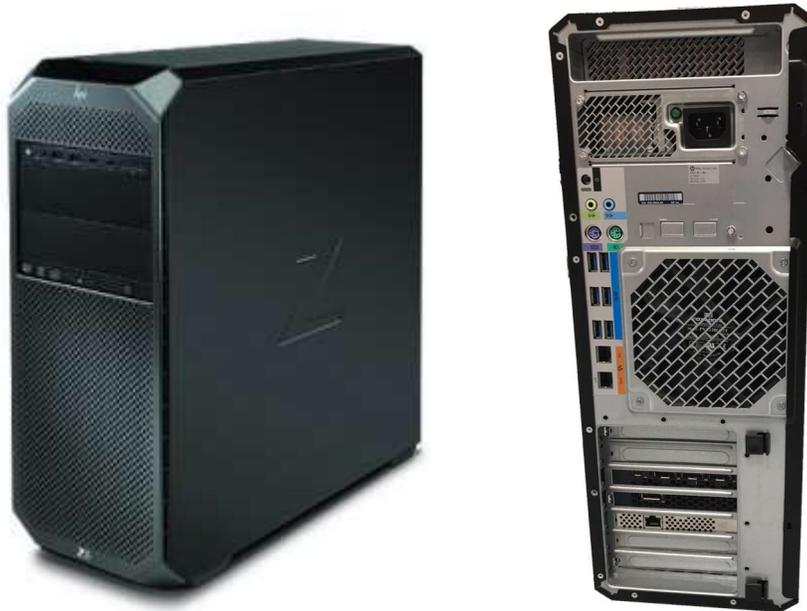
The case can be rack-mounted horizontally using brackets (sold separately). It takes up 4U of rack space. It can be mounted in rack-ready servers cabinet compliant with the EIA 310-D Standard.
