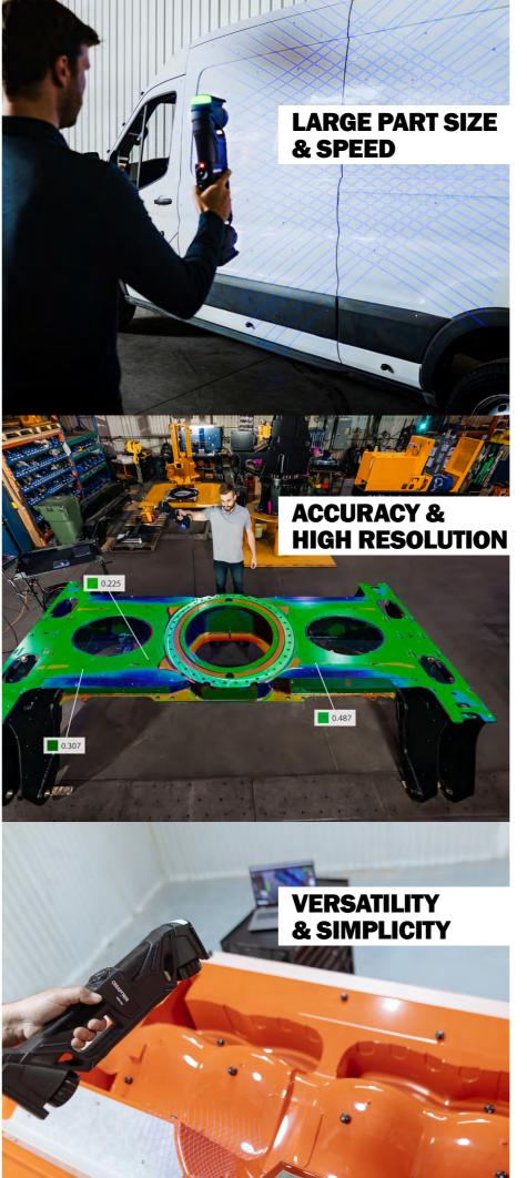
Due to its 38 laser lines and large scanning area, the HandySCAN 3D|MAX Series is the 3D scanner for measuring large part sizes—up to 15 m—quickly and easily, providing metrology-grade results in mere minutes.
